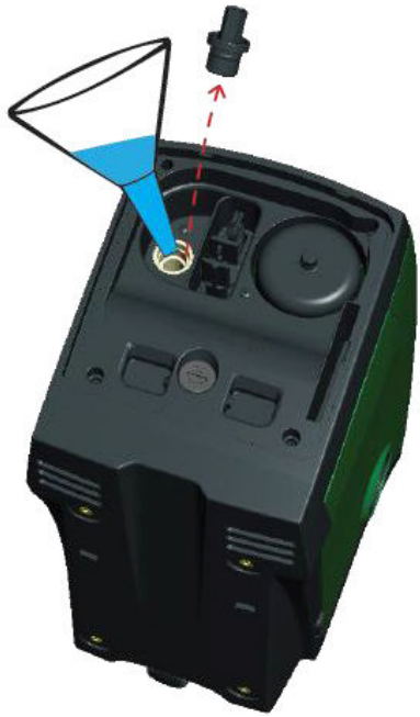
First time water fill up
