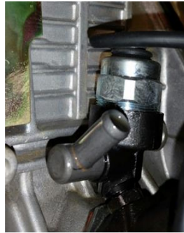
Injector pump inlet
