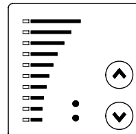
Fig. 12 Control panel of a TPE pump
